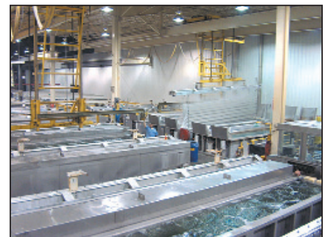
A sophisticated, computerized hoist system guides material through the anodize process
